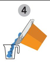
Measure the water collected in the empty container (or pot lined with a bag) to find the total irrigation applied
